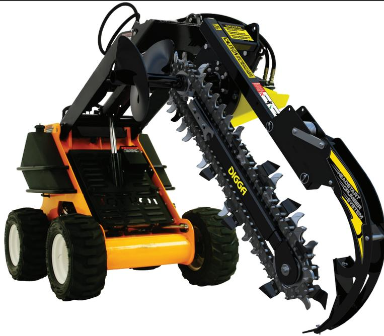
Designed specifically for mini loaders and walk behind machines, the Digga Mini Bigfoot Trencher is the lightest, most compact, powerful mini trencher on the market today. Unique design gives the operator consistent digging depth, efficient spoil to one side of the trench and finely crumbed spoil for effective compaction back into the trench. Provides minimal ground disturbance to surrounding conditions and a cleaner job finish.
